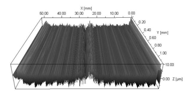
The waviness profile exists twice with evaluation lengths of 25 mm each. This serves to evaluate the Wsa parameter according to SEP1941.
